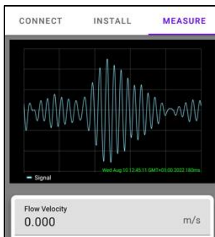
Figure (17) Non-ideal Sensor Positioning, transducers too far apart.
