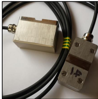
Figure (20) PEEK/stainless steel transducers.
