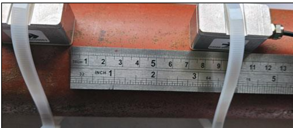
Figure (10) Flow transducer mounting, spacing is 70 mm between front faces.
