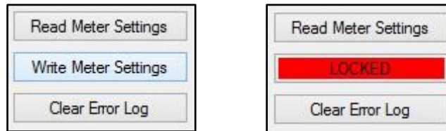
Figure (10) Write meter locked when totaliser is running.
