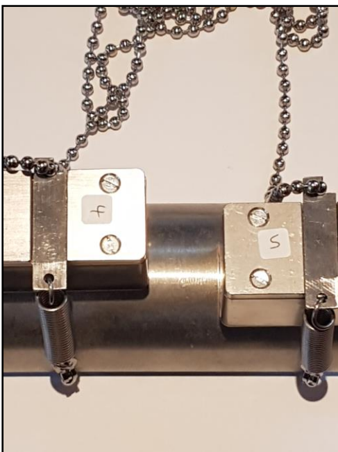
Figure (7) Misaligned transducers.
