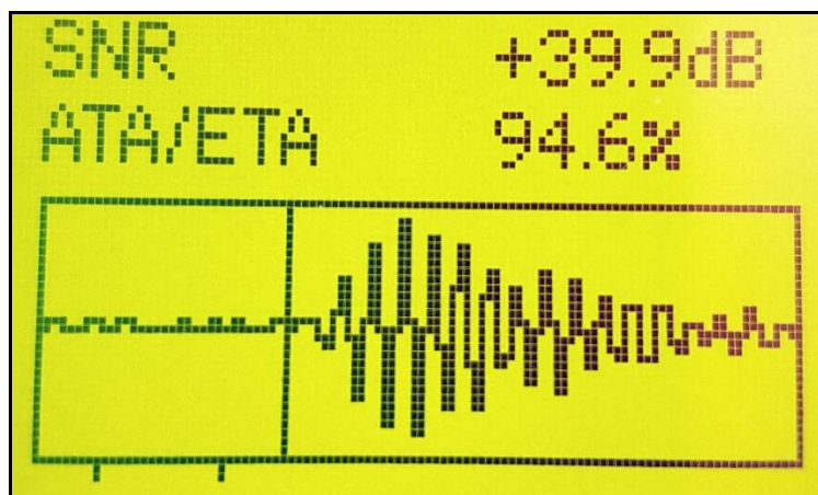
Figure (13) Non-ideal Sensor Positioning, transducers too far apart.
