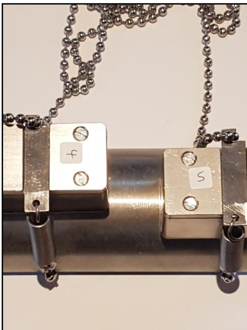
Figure (7) Misaligned transducers.
