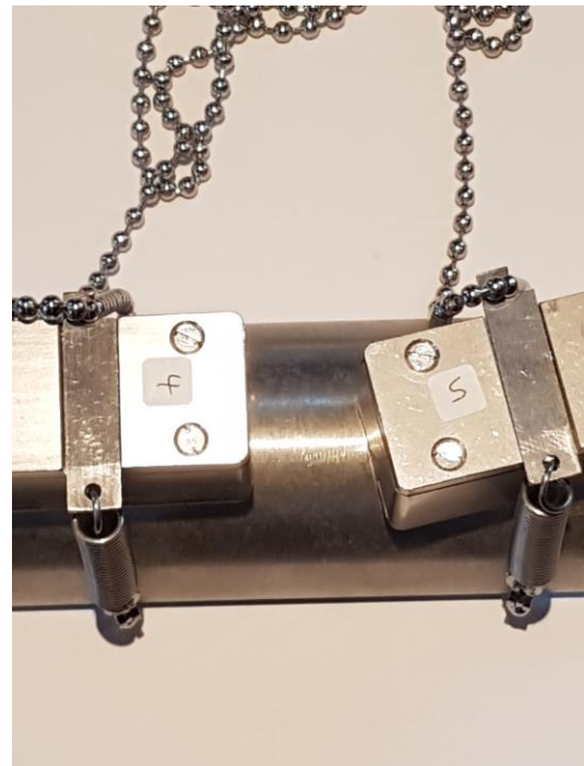
Figure(6) Twisted transducers.
