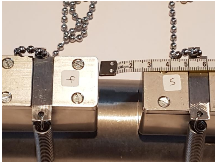
Figure(4) Flow transducer mounting, spacing is 25mm between front faces.
