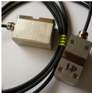
Figure(16) PEEK/stainless steel transducers.
