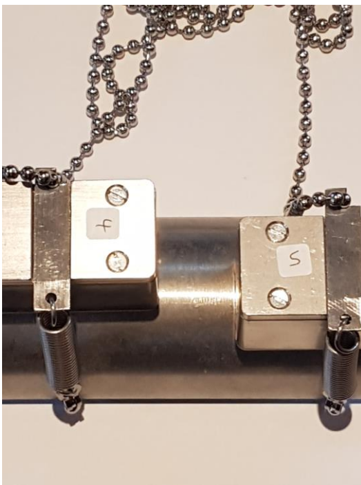
Figure(5) Misaligned transducers.
