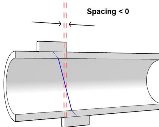
**Figure(6) 1 pass, demonstrating a negative transducer spacing.**
