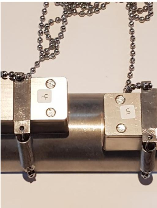
**Figure(4) Misaligned transducers.**
