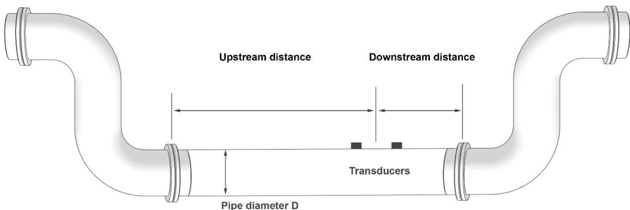
**Figure(12) Upstream and downstream pipe lengths.**
