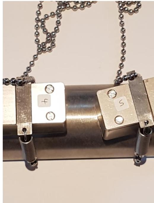
**Figure(5) Twisted transducers.**
